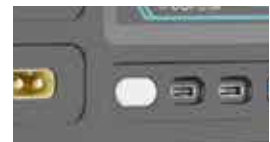
4. Type-C, PD 100W fast charge
